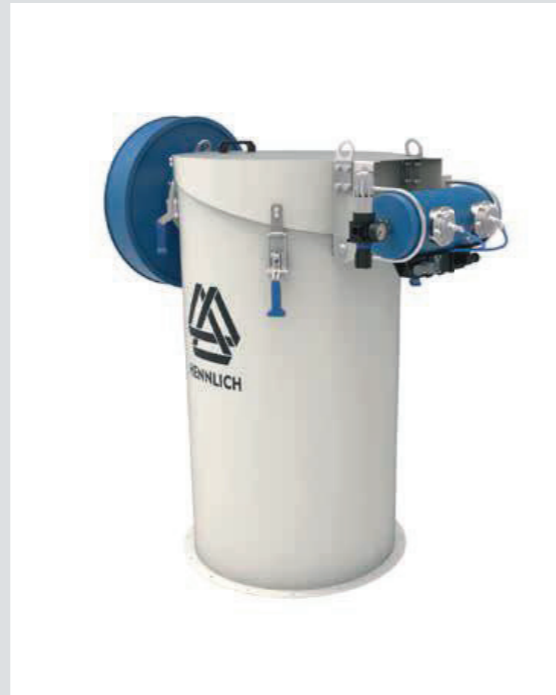
Silo venting filter NH1000 V is a cylindrically shaped dust collector. It is mainly used for dedusting of silos and for local filtration.
